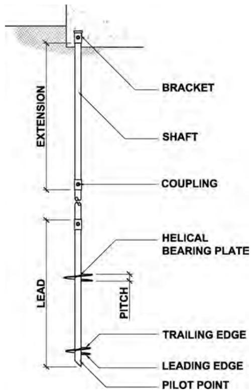
**Figure 1.1 Basic helical pile**
