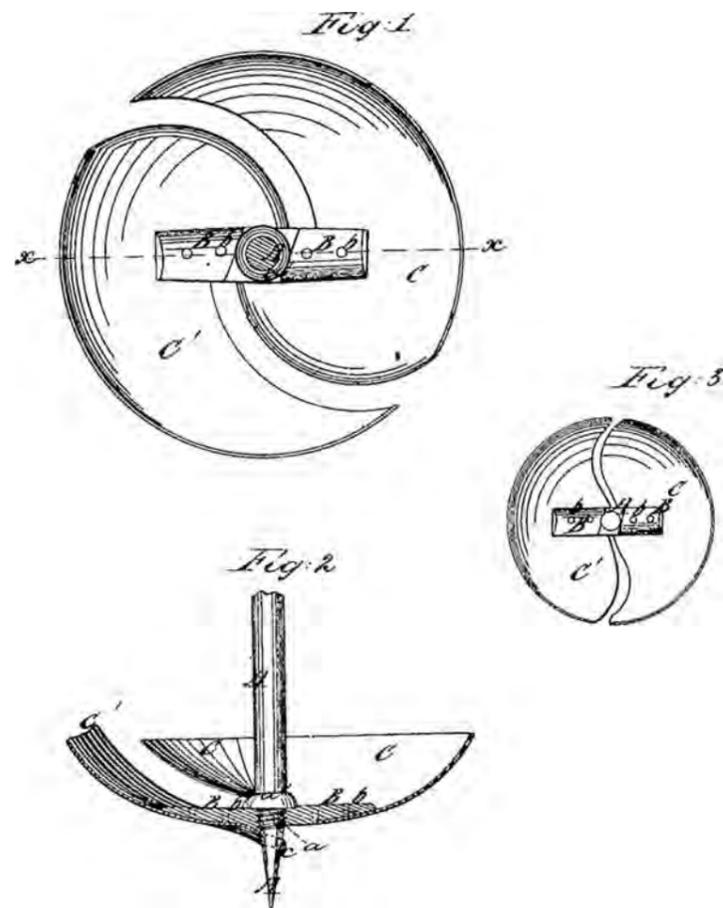
**Figure 1.10 Ballard earth-borer device**
