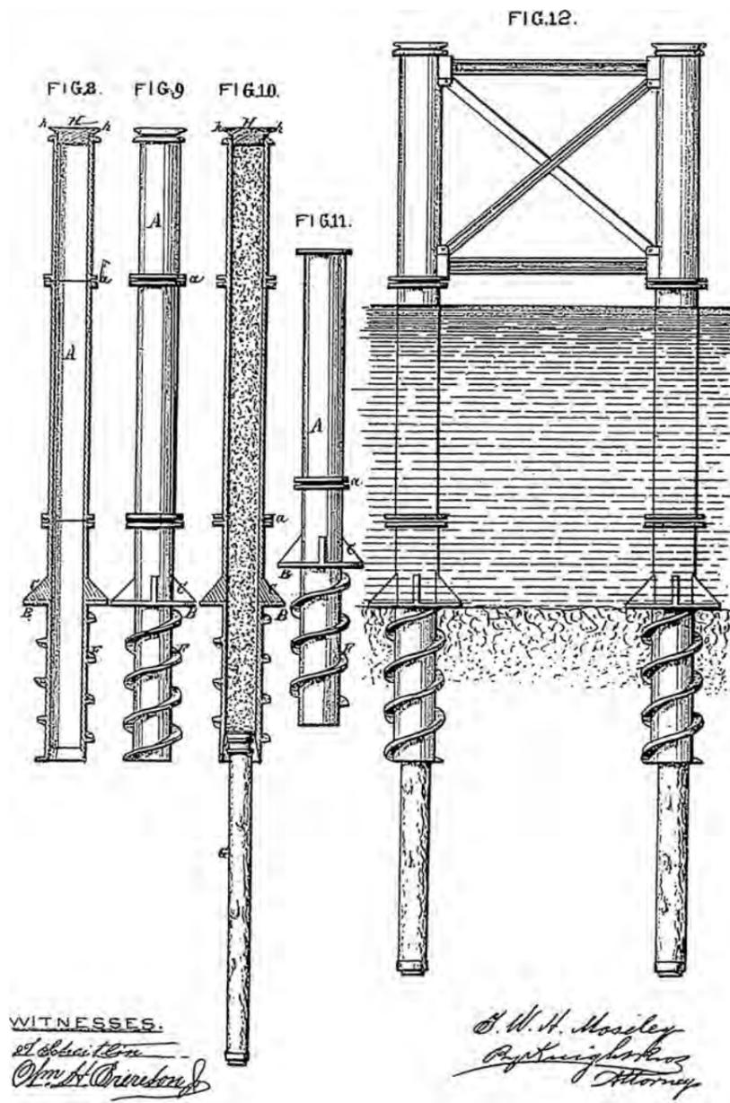
Figure 1.8 Moseley helical pile patent (Cont.)
