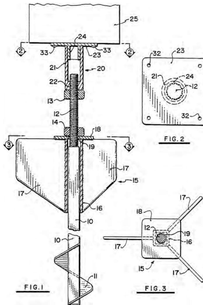
Figure 1.15 McFeeters lateral stability device
