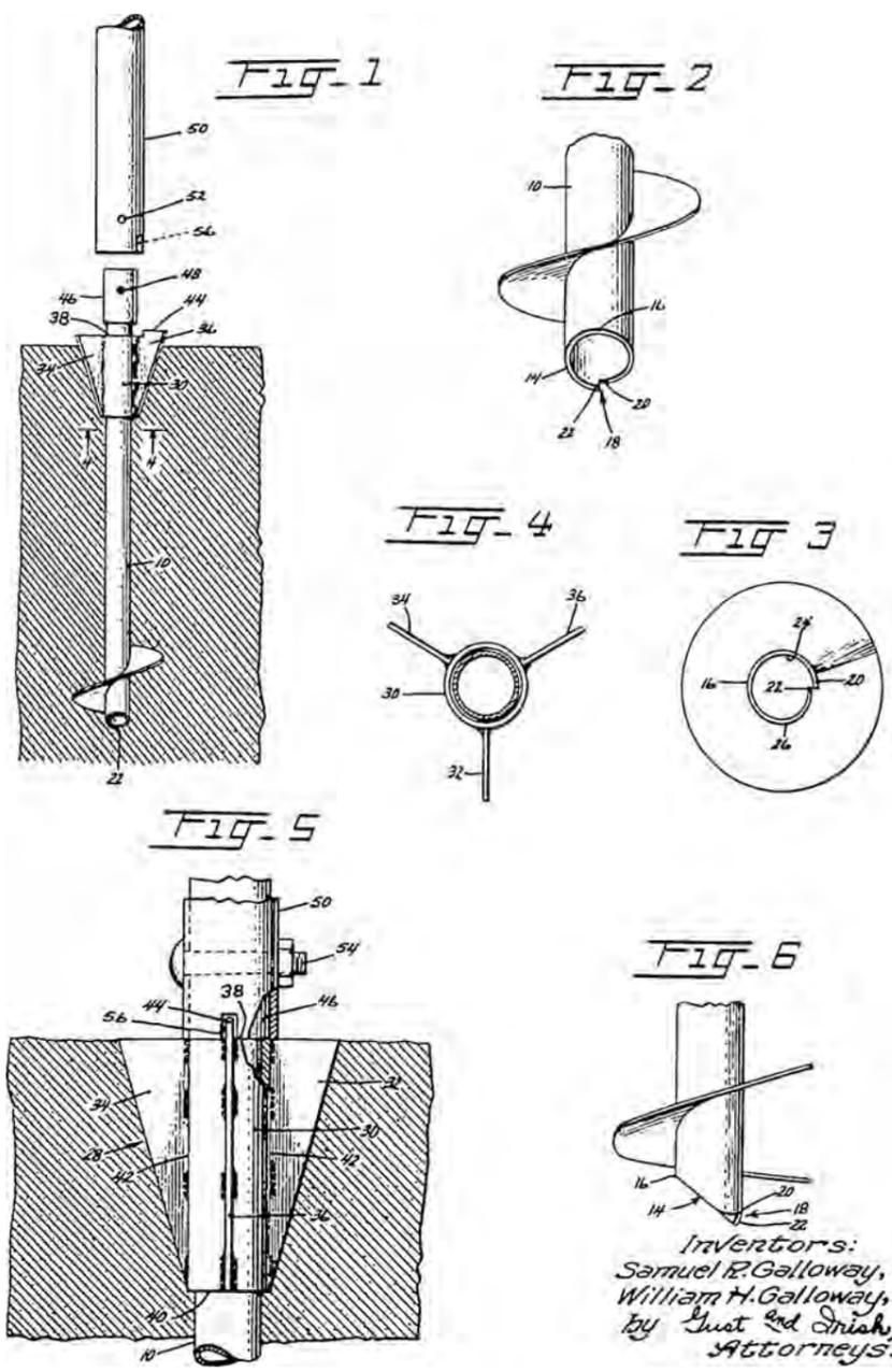
Figure 1.14 Galloway lateral stability device
