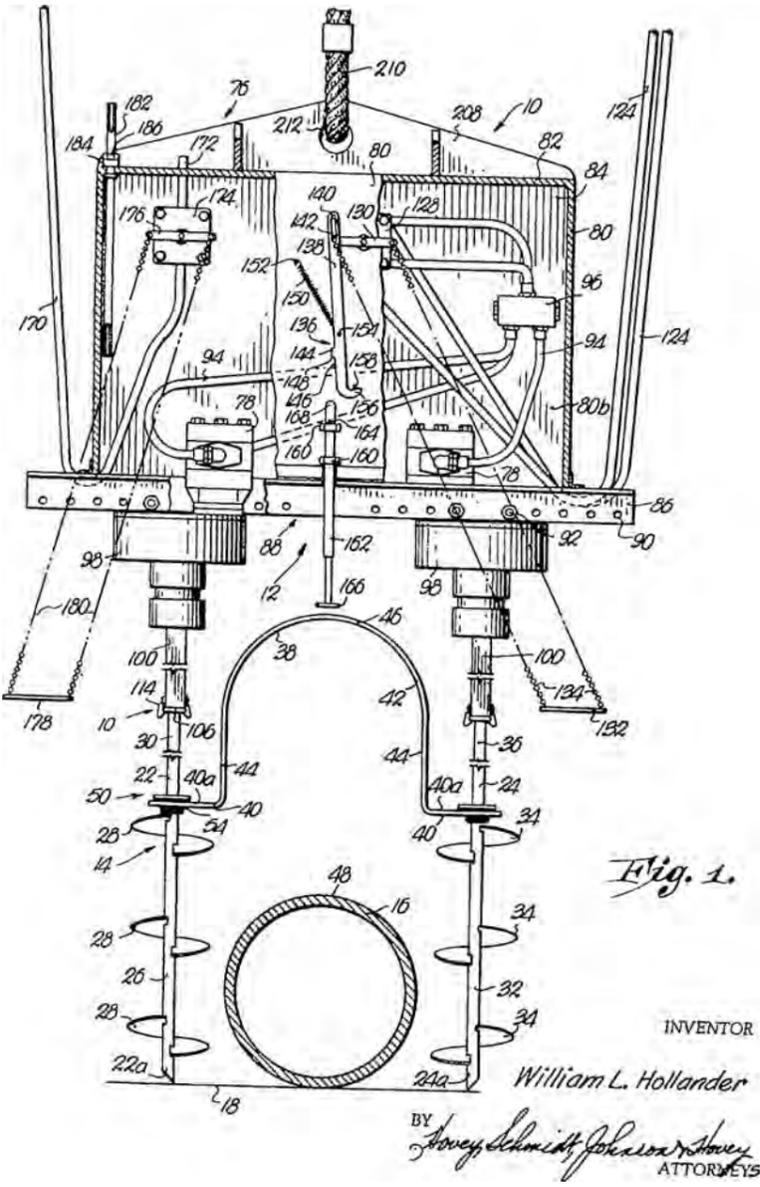
Figure 1.12 Hollander pipeline anchor installation method
